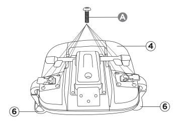
**Tip:** For easier installation, place seat on top of box. Hand thread all screws prior to fully tightening with T-wrench.
