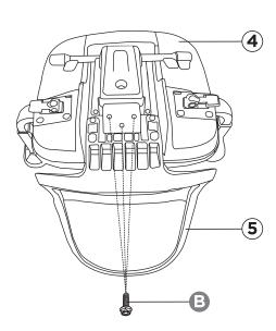
**Tip:** Hand thread all screws prior to fully tightening with T-wrench.
