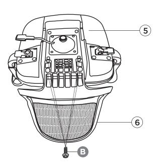
Tip: Hand thread all screws prior to fully tightening with T-wrench.
