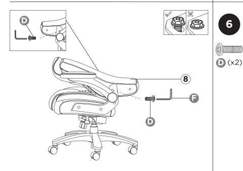
**Tip:** Use Allen wrench to thread all screws. Do not tighten screws fully until you have complete assembly. **D** (x4)
