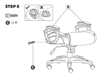
**TIP:** Use Allen wrench to thread all screws. Do not tighten screws fully until you have complete assembly.
