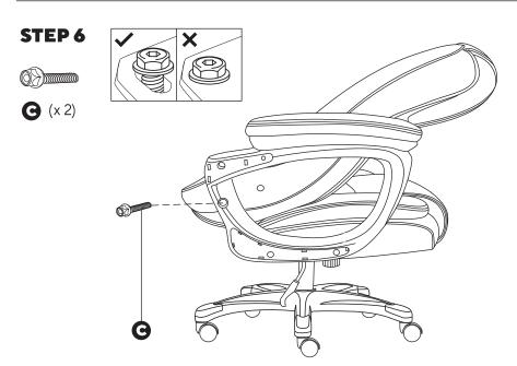
**TIP:** Use Allen wrench to thread all screws. Do not tighten screws fully until you have complete assembly.
