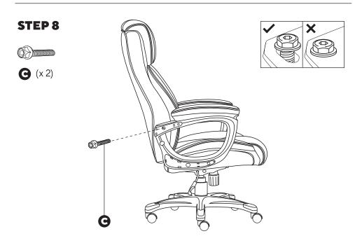
**TIP:** Use Allen wrench to thread all screws. Do not tighten screws fully until you have complete assembly.
