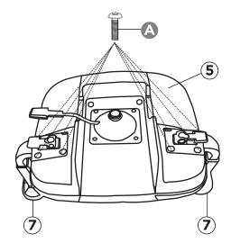
**Tip:** For easier installation, place seat on top of box. Hand thread all screws prior to fully tightening with T-wrench.
