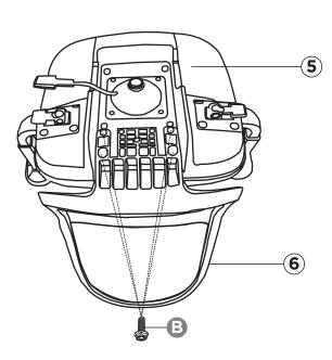
**Tip:** Hand thread all screws prior to fully tightening with T-wrench.
