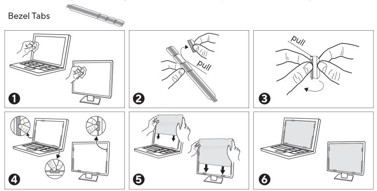
Place the bezel tabs along the raised edges of the sides of your screen.
