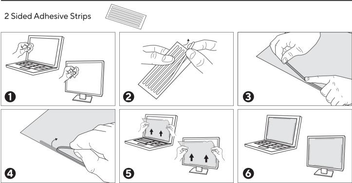
Position the adhesive strips as close to the edge of the filter as possibility to minimize their visibility on the screen. The number of adhesive strips needed may vary depending on screen size.
