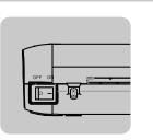
Ensure temperature switch on side of machine is set to on. Wait for green light.
