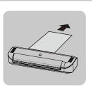
To prevent jamming, immediately remove laminated item from back of machine. Let item cool on flat surface for several seconds
