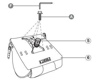
**TIP**: For easier installation, place seat on top of box. Hand thread all screws prior to fully tightening with Allen wrench.
