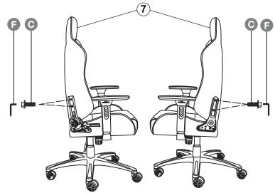
**TIP**: Hand thread all screws prior to fully tightening with Allen wrench.
