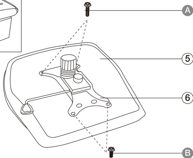
Tip: Hand thread all screws prior to fully tightening with allen wrench.
