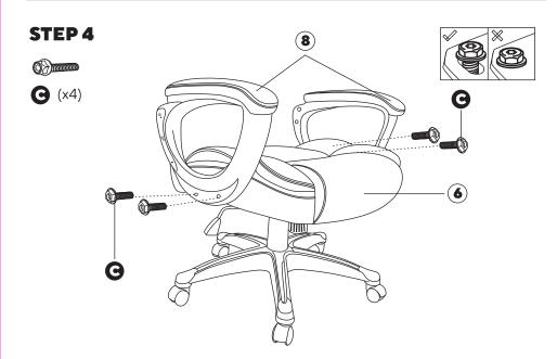
**TIP:** Use Allen wrench to thread all screws. Do not tighten screws fully until you have complete assembly.
